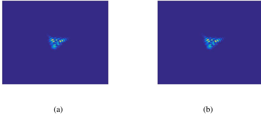
Figure 4.1. (a) Synthetic PSF created from modeled phase errors. (b) Output PSF estimate from the PR algorithm.
